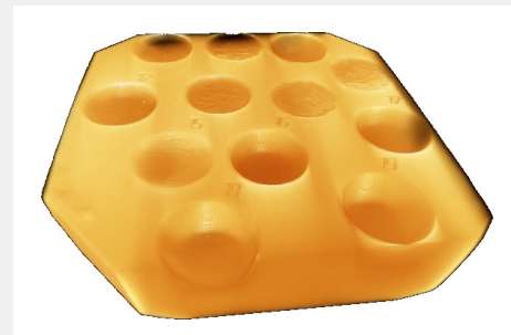
3D image of a lens array produced in a cheap yellow diamond.
