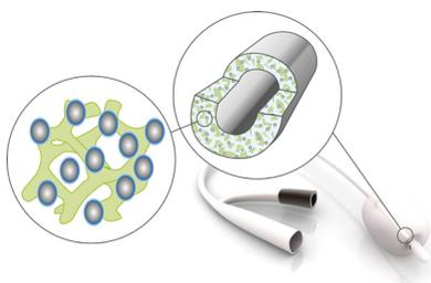
Soaking Biomodics IPNs in heavy water ( $D_2O$ ) highlights the hydrogel structure when analysed with neutrons. This enables a determination of characteristic sizes from the SANS data. One important parameter is the chord length, which is a measure of the average size of the hydrogel domains.
