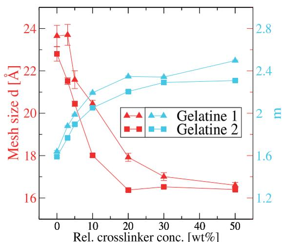
The obtained SAXS curves show a variation with increasing amount of cross-linker in the binder material. With more cross-linker, the mesh size of the binder decreases until a concentration of about 20%. This is correlated to functional properties of the final stone wool product.
