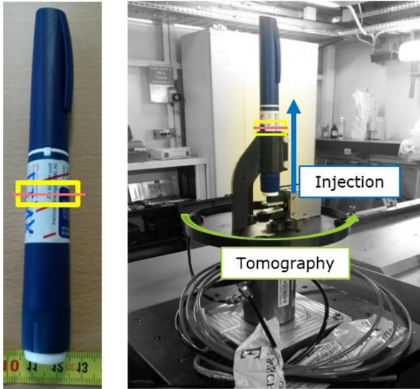
Insulin pen set-up for CT scanning under operation.
