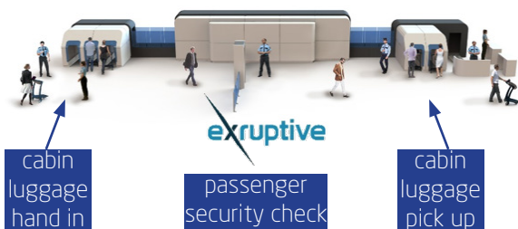
Schematic representation of the security solution offered by Exruptive. A trolley is loaded with the cabin luggage and passes its way through the scanner system, while the passengers have the security check. There is no need for divesting the luggage.
