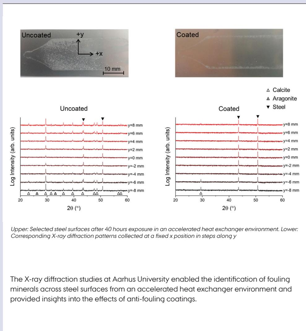
Upper: Selected steel surfaces after 40 hours exposure in an accelerated heat exchanger environment. Lower: Corresponding X-ray diffraction patterns collected at a fixed x position in steps along y
